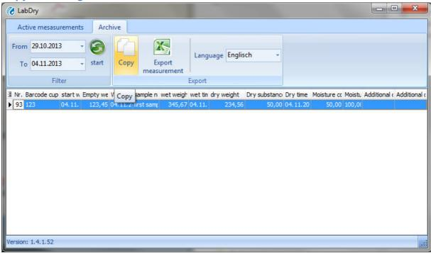
Pressing the button "Copy" all selected measurements are transferred into the clipboard. This data incl. headline is now available for further analysis.
