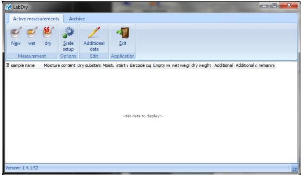
After successfully transferring the dry weight, the measuring data is switched to the archive. From now on the bowl can be used for measuring a new sample!
