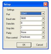
Please check the right interface number in the device manager of your windows programme (system control -> system -> hardware -> device manager -> connections)
