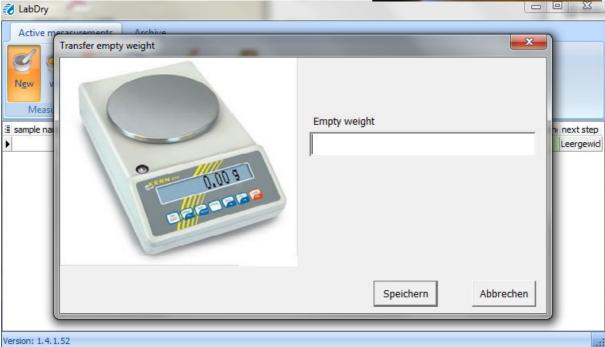
After reading the barcode a new popup window asking for the empty weight appears. For that, place the empty and clean bowl at the centre of the scale.
