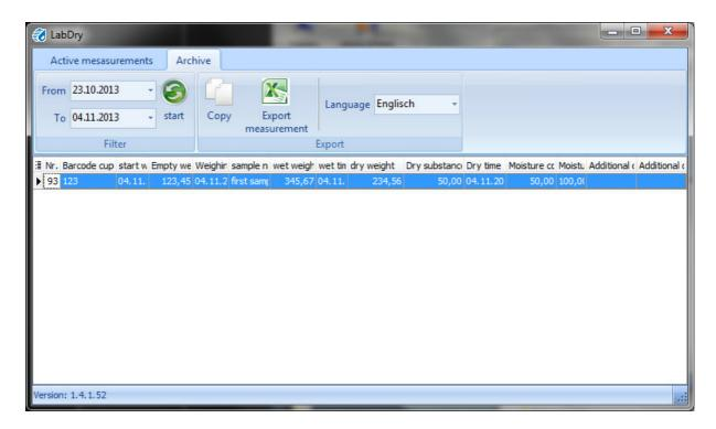
Now all measurements in the desired time period are displayed. Note that the archive contains all completed measurements, even when they are currently not shown on the display.
