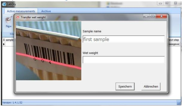
Now press the button "wet". A popup window asking for the barcode appears. Scan the barcode of the bowl using the barcode scanner. After the successful scan a new popup window asking for the sample name and wet weight appears. Please enter a sample name now. The entered name can be modified afterwards.
