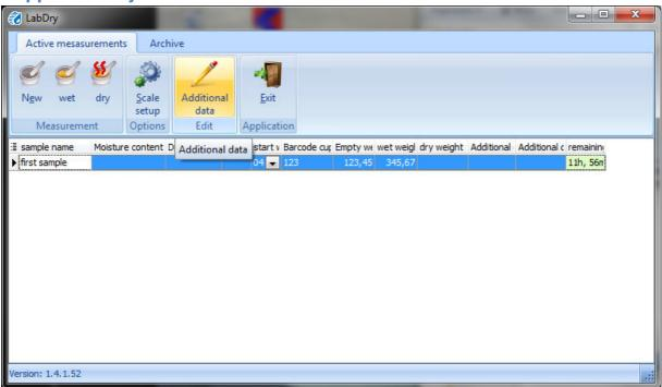
When the wet weight has been entered, you can insert additional information about this sample. Also the sample name can be modified now. This is the last time that supplementary data and sample name can be added or changed.
