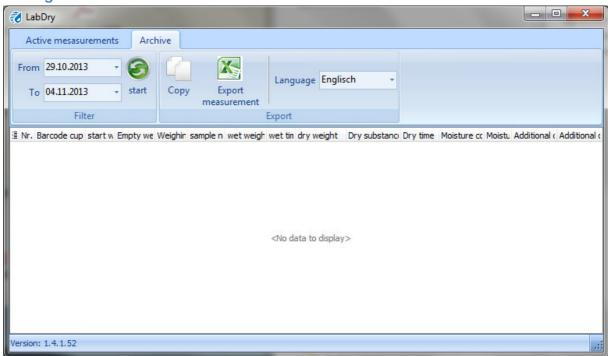
For ensuring a well-arranged and clear view of completed measurements, you have to select a certain time period of measurements that should be shown. After entering the date and pressing the "Start" button the respective measurements are displayed.
