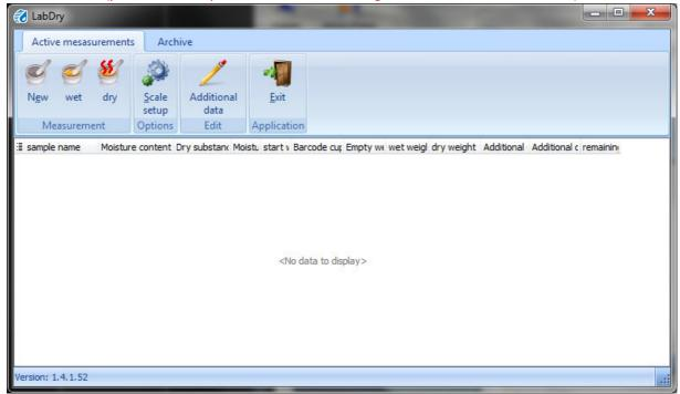
This window represents the main menu. The programme is subdivided into two parts: the tab "Active measurements" and the tab "Archive". All active measurements and already scanned sample bowls are shown in the window "Active measurements". As soon as a sample bowl comes out of the drying chamber and the dry weight is transferred, the corresponding measuring data moves to the archive.
